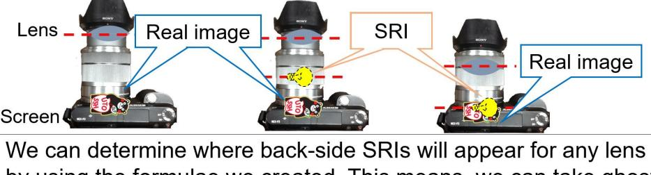
by using the formulae we created. This means we can take ghost photographs by adjusting the distance between the lens and the screen. We can also prevent ghost photographs by using anticoating lenses because it was found that SRIs are formed by internal reflections within a lens [Chap.12] [Fig.3]
