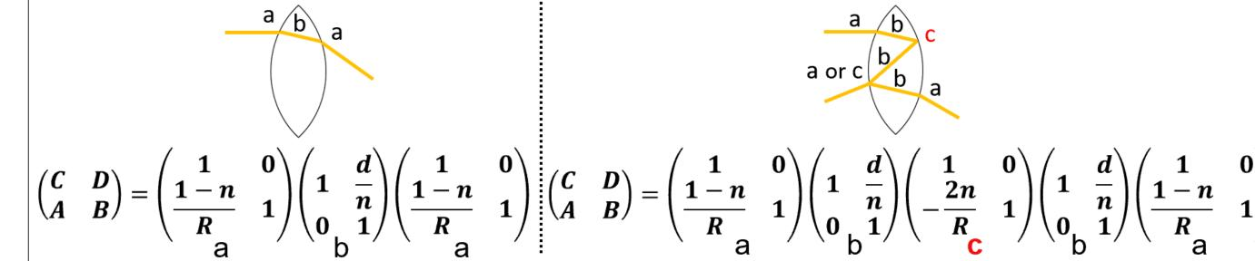
Four formulae for a plane-convex lens were used to locate the positions of SRIs. Two patterns (labeled  $\alpha$  and  $\beta$ ) were investigated in order to check whether the calculation results were same or not. Each results were same, so we thought that we could minimize the calculation mistakes, and improve the accuracy [Chap.5] . The fact that the same results were obtained for both the  $\alpha$ - and  $\beta$ -patterns confirmed the robustness of the formulae.
