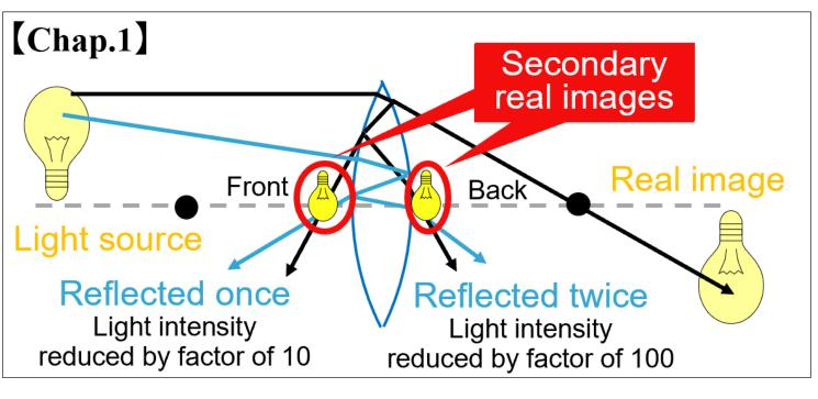
Previous research has shown that there are two more small images formed at the front and the back sides of a convex lens, which are known as secondary real images (donated by a SRI or SRIs). These are produced by internal reflection of light rays within a lens that is not parallel to the optical axis [Chap.1].
